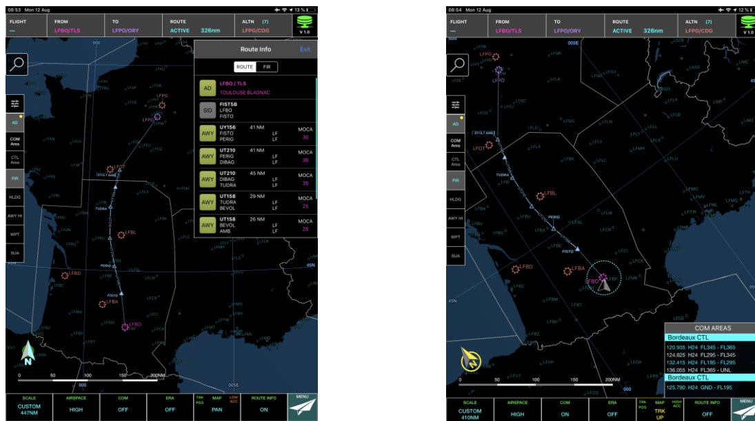
Figure 1: Enroute (Home) screen populated with departure, arrival, alternate and route parameters (left) and with own-ship position in Track up mode (right)
